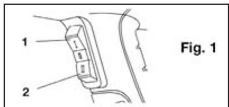
The Heat Gun has a 3-position trigger switch that acts as both an ON/OFF switch and a temperature selector switch (Fig. 1).
